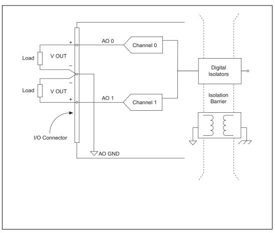
Figure 5-2. Analog Output Connections
